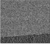
This is a scanning electron microscope image of a WC-17 Co coating applied by kinetic metallization on 4340 steel.
